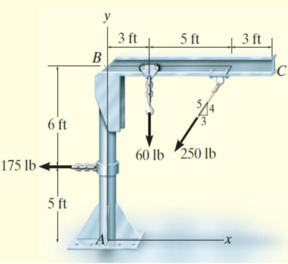
**Find:** The equivalent resultant force and couple moment at the origin O. Also find the location (x, y) of the single equivalent resultant force.
