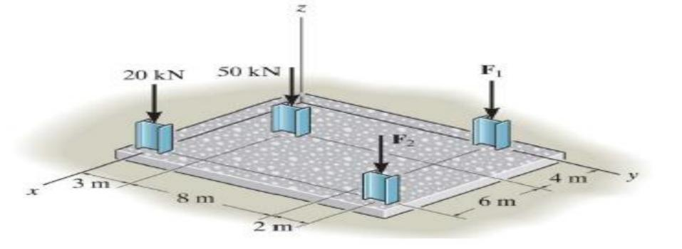
$F_1 = -20 k & \& F_2 = -50 k \\ r_1 = 10 i & \& r_2 = 4i + 3 j \\ F_{RO} = -20 k - 50 k = -70 k \text{ KN}$
